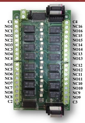
The operating condition of the contacts marked on the board (NC, NO) refers to the relay at rest, if the relays are energized condition of operation is reversed
