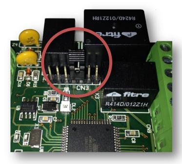
**N.B.:** You can restore the default settings (IP = 192.168.1.222) by shorting pin 3 to pin 4 of connector for programming the board CA230. Wait a couple of seconds, turn off and remove the short. The next time the system will have the default configuration.
